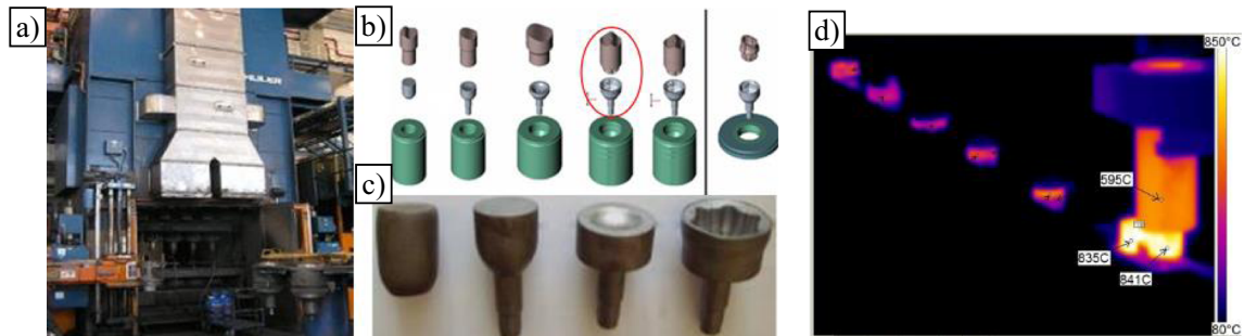
Fig. 2 The precision forging process. a Crank press. b Scheme of individual operations (V operation—marking). c Forgings after successive operations. d The thermovision research
