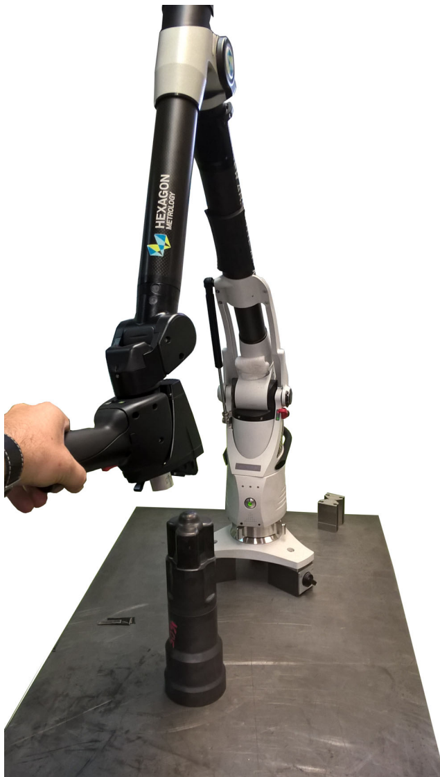
Fig. 5 A forging selected for the analysis during scanning on the measuring station
