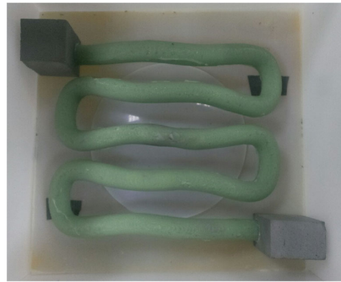
Fig. 2 Placement of positioning fixtures and conformal cooling channel in the mold frame
