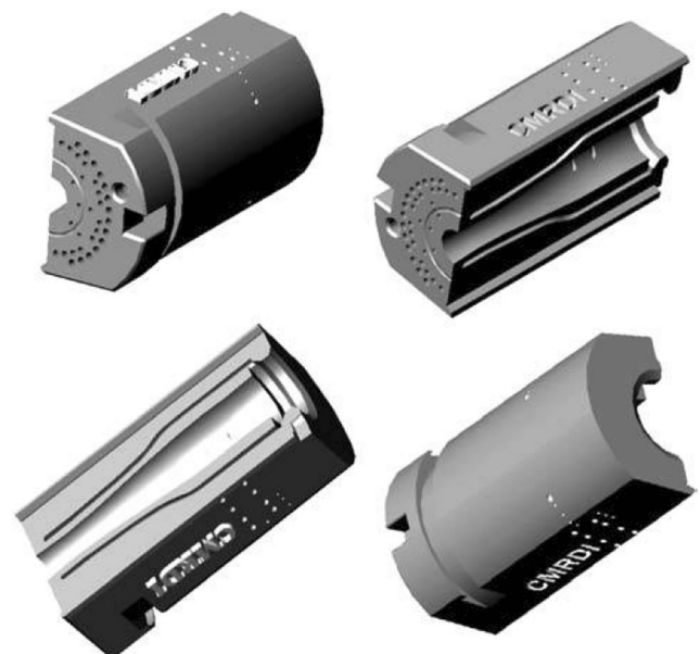
Fig. 26 Benchmark artifact proposed by Abdel Ghany and Moustafa [38] (overall dimensions = 200 mm × 100 mm × 40 mm)
