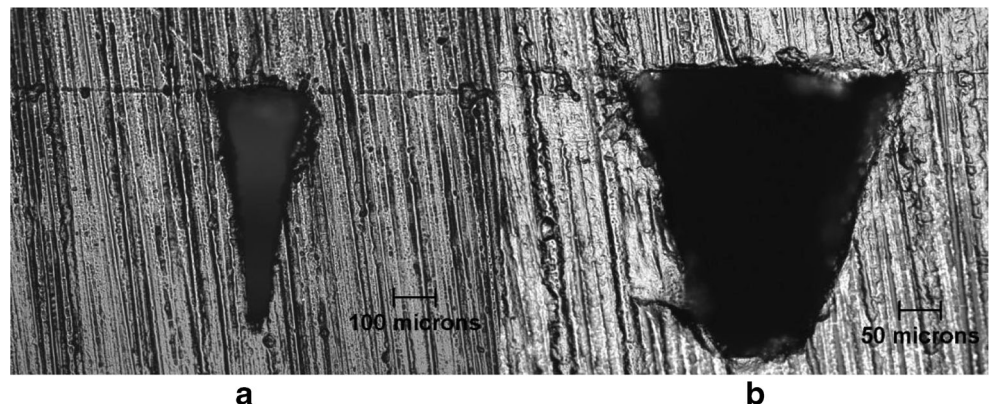
Fig. 26 Profile of the a triangular and b trapezoidal microchannels after thermal bonding
