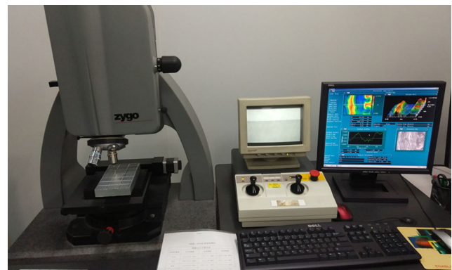
Fig. 12 Zygo NV5000 surface topography interferometer
