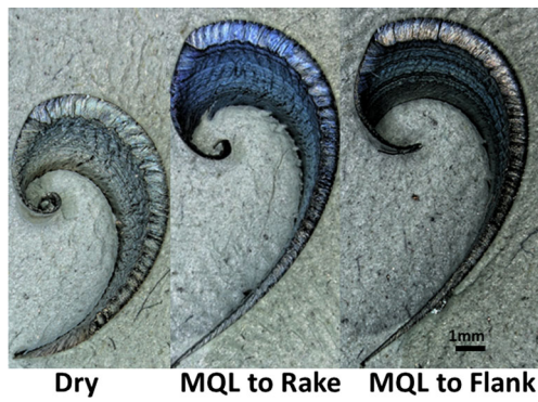
Fig. 7 Shape of the chips after different machining environments
