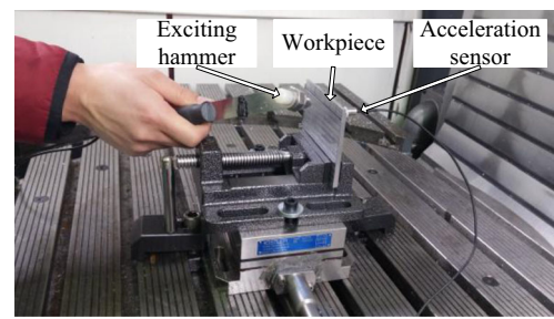
Fig. 4 The modal test experiment
