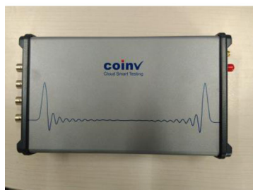
(b) The INV3062T type four channel data acquisition instrument
