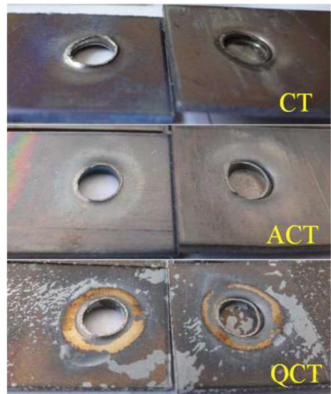
Fig. 8 Failure modes after tensile–shear tests
