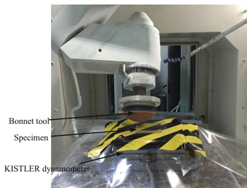
Fig. 9 Measurement of the forces in the polishing process by 3-component dynamometer
