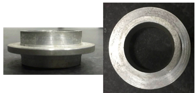
Fig. 12 The AL_2017 blank with a radial step
