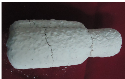
Fig. 16 Cracked shell due to increased percent of additives
