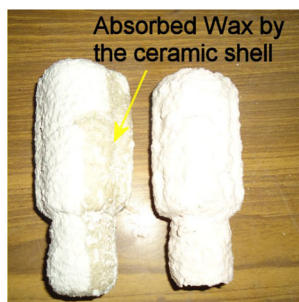
Fig. 4 Ceramic shell absorbed wax from wax pattern during dewaxing
