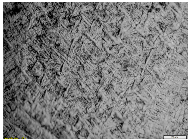
Fig. 4 Micrographs showing the microstructure of samples produced at a scanning speed of 0.06 m/s and powder flow rate of 0.72 g/min, b scanning speed of 0.06 m/s and powder flow rate of 6.48 g/min
