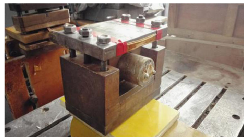
Fig. 3 Magnetic pulse welding setup with UPEA
