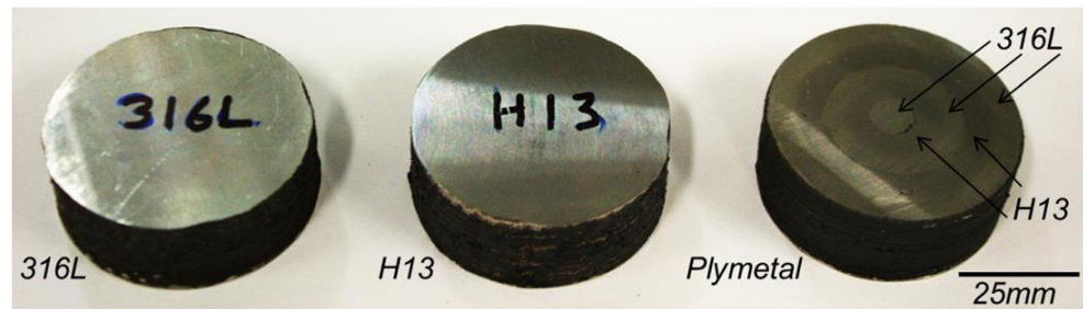
Fig. 3 Samples after manufacturing by laser-assisted direct metal deposition. Alternating metals are visible in plymetal sample
