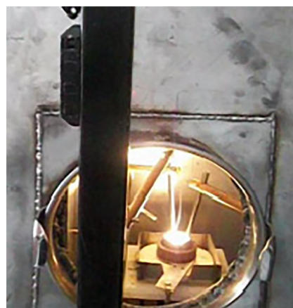
Fig. 1 A photograph of the homemade electric arc furnace
