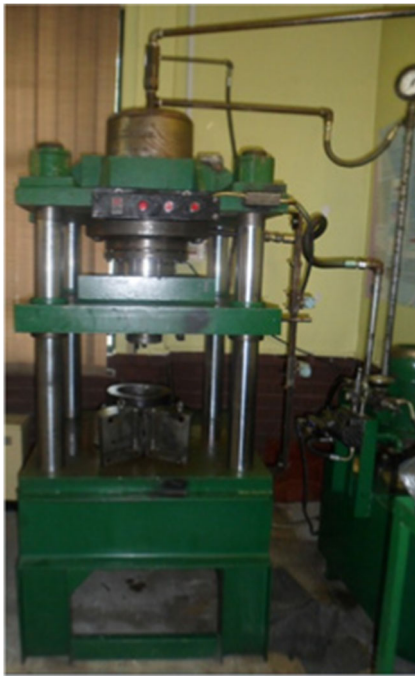
Fig. 4 Used hydraulic press of 200 t nominal capacity
