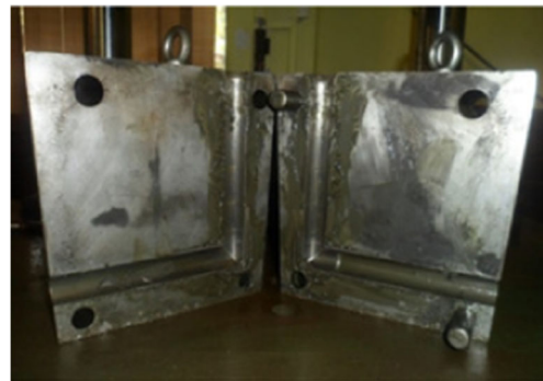
Fig. 3 The used ECAP die with channel diameter of 20 mm and channel angle and corner angle of 90° and 20°, respectively
