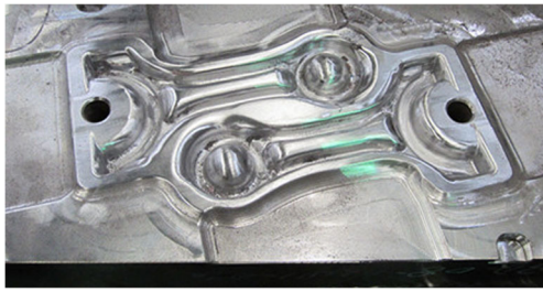
Fig. 5 Top die of the pre-forging process for connecting rods
