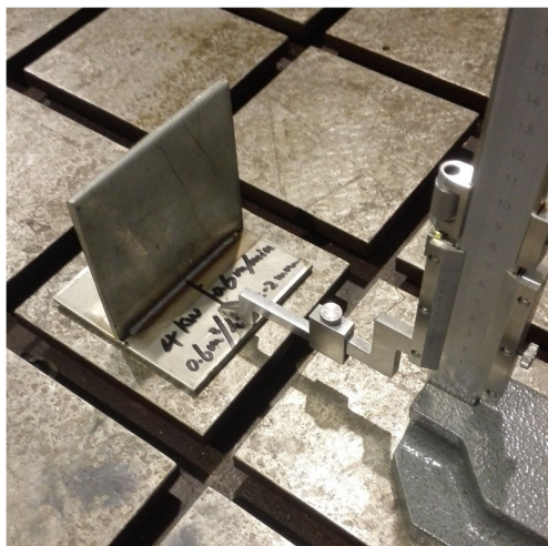
Fig. 8 Measurement method of angular distortion
