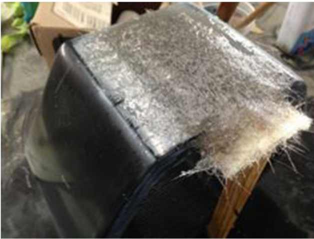
Fig. 5 Fiberglass composite cured on a planar mold
