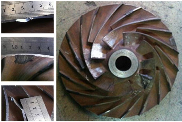
Fig. 1 Failure open impeller
