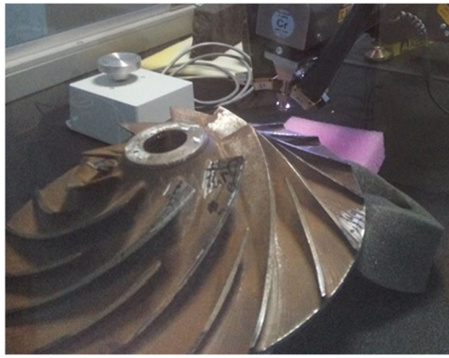
Fig. 10 Residual stress measurement by XRD
