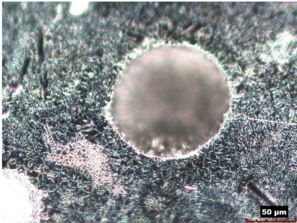
(a) Optical Image of Gas Porosity
