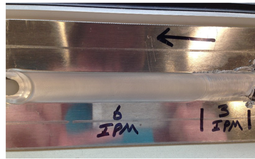
Fig. 7 Top side of a sample weld
