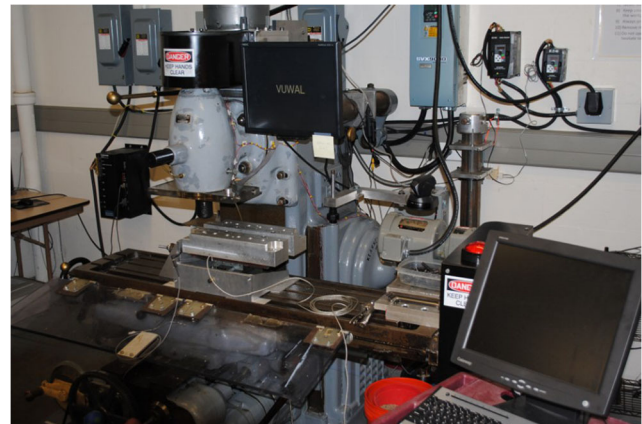
Fig. 2 FSW machine used for the development of the SAA-FSW tool
