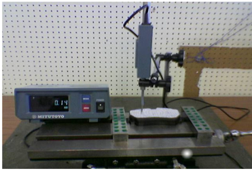
Fig. 26 An arrangement of brake pad surface measurements
