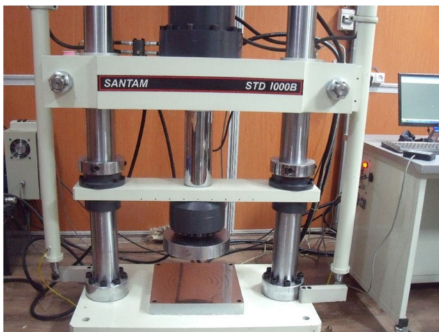
Fig. 12 Applied stamping device as acting force in the die
