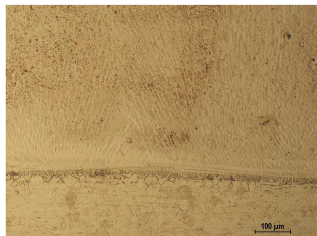
Fig. 8 Micrograph of marage (upside) and AISI 304 (downside) interface
