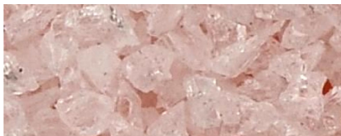
Fig. 1 Dominating noble electrocorundum 56A abrasive grain shapes [1]
