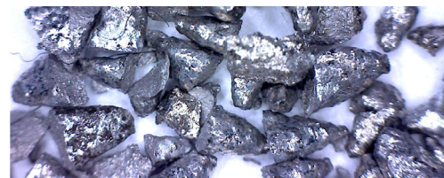
Fig. 2 Dominating abrasive grain shapes in aluminium oxynitride 55N—ABRAL© [1]
