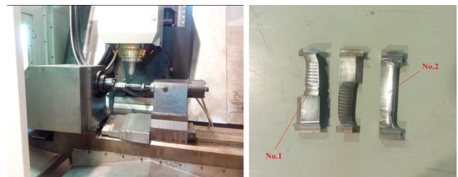
Fig. 10 The five-axis machining center (XKH800) and workpieces of various types used for machining
