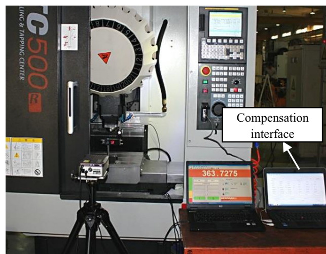
Fig. 10 Experimental compensation verification test
