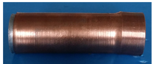
Fig. 10 Al-Cu composite tube subjected to longer ball spinning stroke
