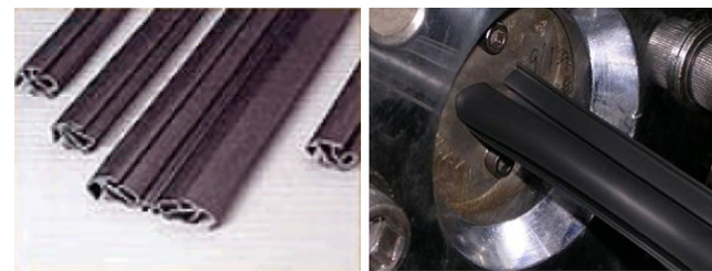
Fig. 1 a Weather strips used for vehicles, b real forming scene
