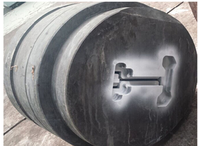
Fig. 11 Extrusion die assembly used in experiment
