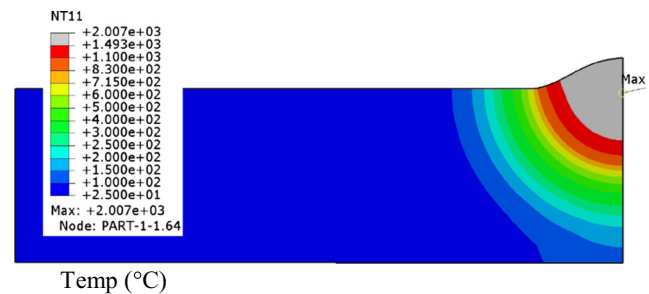
Fig. 13 The 2D axi-symmetric model and predicted temperature distribution of the fusion zone
