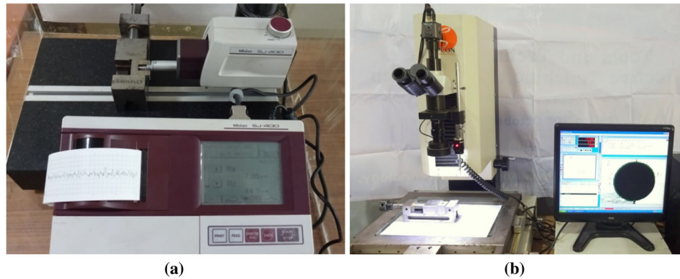
Fig. 7 Measuring equipments. a Surface roughness tester. b Vision measurement system
