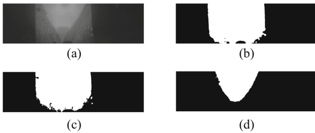
Fig. 4 Comparison of the image-processing results of the welding pool region for three different threshold-selection methods. a Original image. b Average-gray-value threshold-selection method. c Otsu automatic threshold-selection method. d Threshold-selection method developed in the present study
