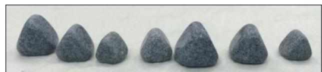
Fig. 7 Straight-cut triangular ( F -triangle) ceramic media used
