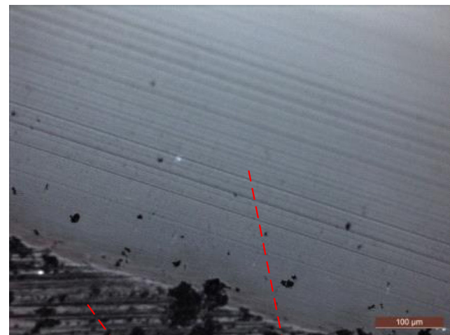
Fig. 10 Microscope image of the machined surface after grinding and semi-finish fly cutting
