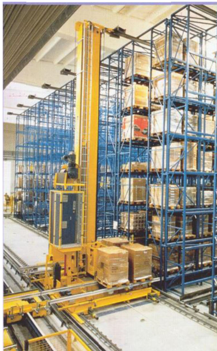
Fig. 1 Multi-aisle AS/RS with aisle transferring S/R machine
