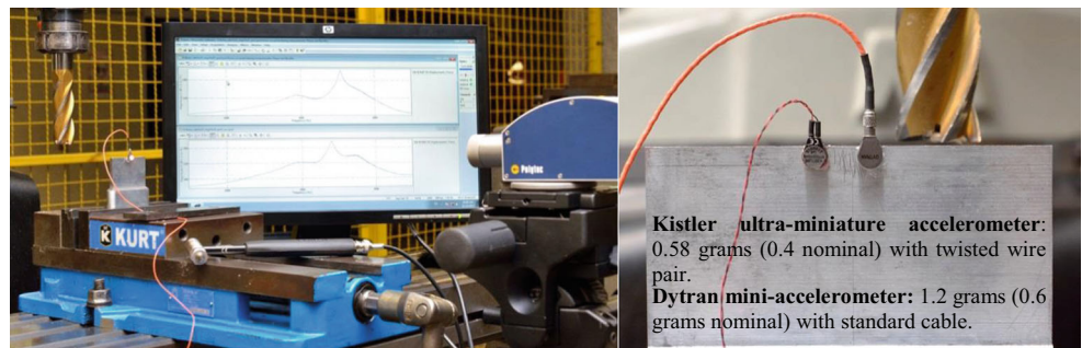
Fig. 4 Left: experimental setup for FRF measurements using LDV and accelerometer devices. Right: Kistler ultra-miniature accelerometer and Dytran mini-accelerometer attached to a thin wall of 1 mm thickness
