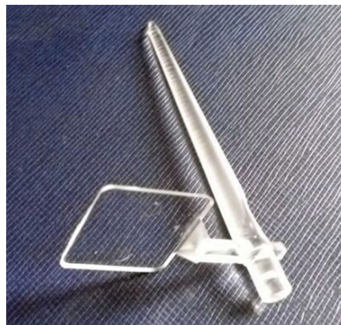
Fig. 11 PMMA injection-molded nanopillar array with its runner system
