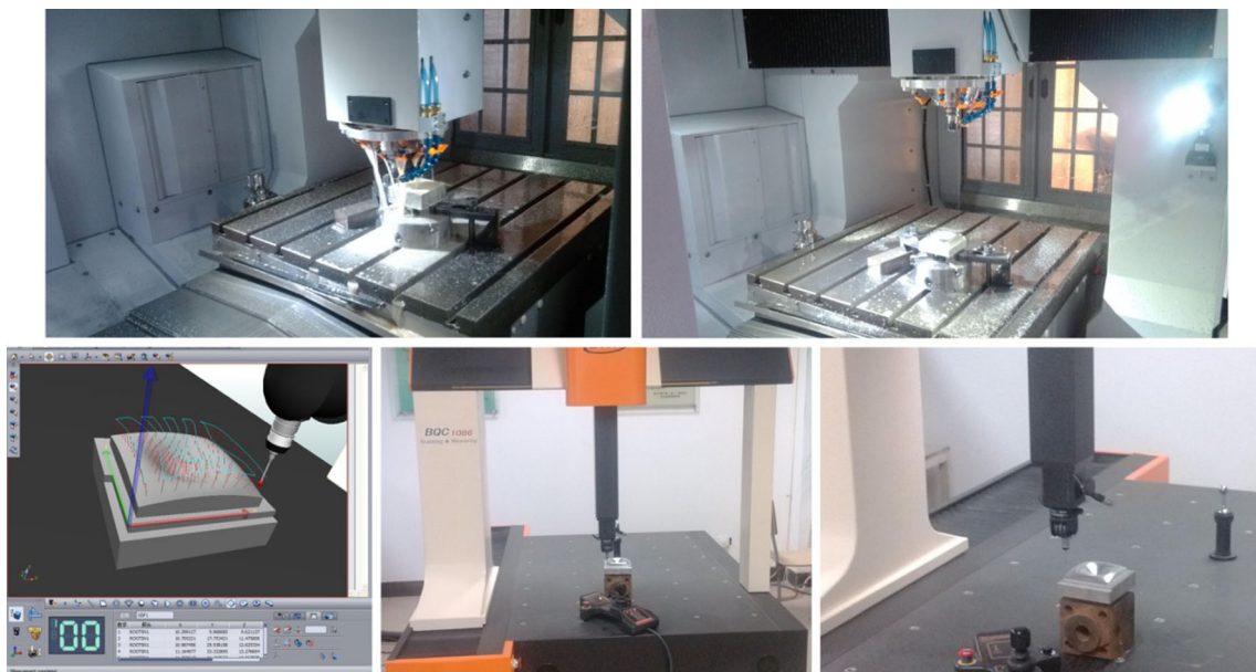
Fig. 10 The machining on the machine tool and the measurement with CMM
