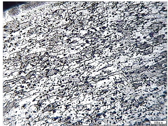
Fig. 11 Microstructure of the formed region of the OFS sample
