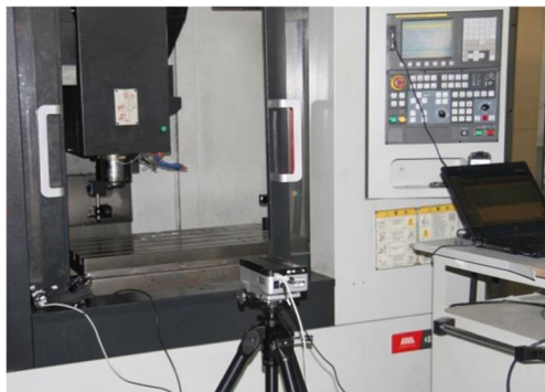
Fig. 5 Test of thermal errors using a laser interferometer
