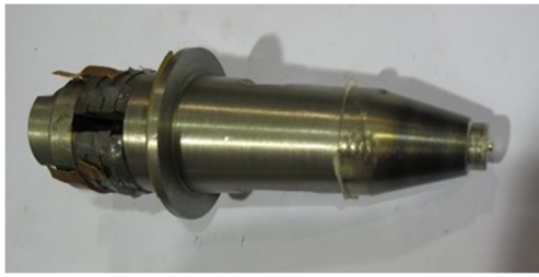
Fig. 5 Assembled FSW vibrational tool and its flange
