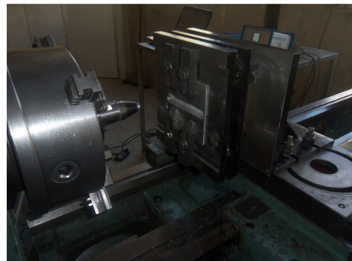
Fig. 8 The vibrational FSW setup on a turning machine
