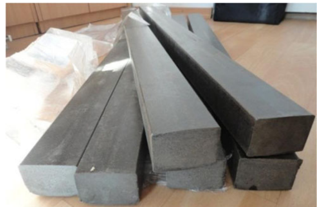
Fig. 1 WPC samples used in the experiment (profiles of 40 \times 60 \times 3,600 mm)
