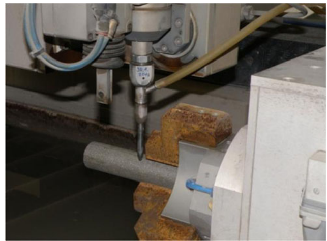
Fig. 4 Samples clamping in chucks before AWJ/WJ turning
