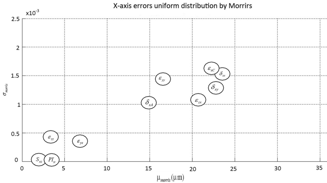
Fig. 12 Uniform distribution of X-axis errors by Modified Morris Method
