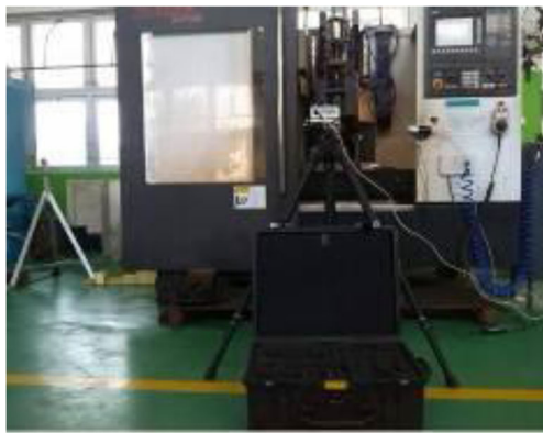
Fig. 3 The measurements setup of error parameters
