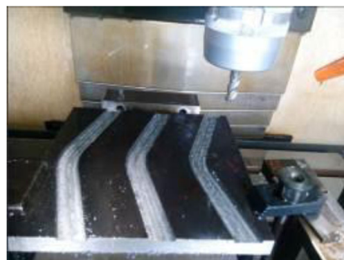
Fig. 5 Milled work pieces under different error compensation scheme
