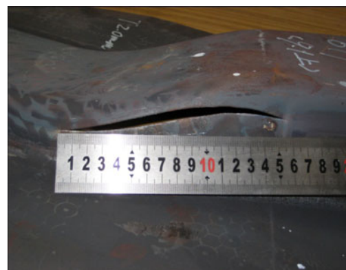
Fig. 13 The experimental final fracture located at the B-pillar
