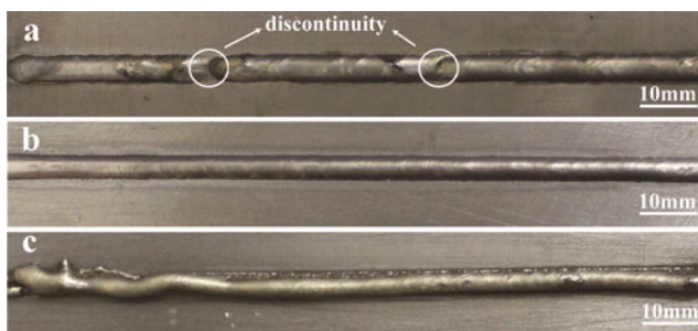
Fig. 5 Typical weld formation under different wire transfer types: a 120 A; b 90 A; and c 20 A: ( P=2 kW, V_f=2 m/min)
