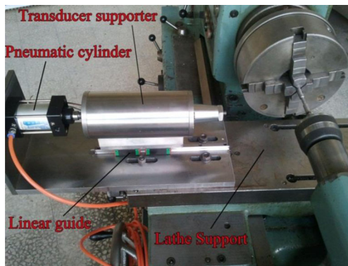
Fig. 5 UNSM fixture assembled on TN50A lathe
