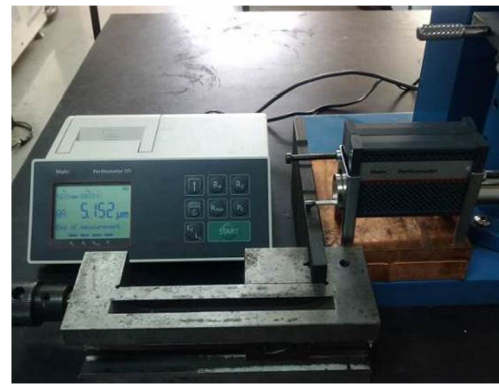
Fig. 2 MAHR-Perthometer M1 instrument for the measurement of machined surface roughness
